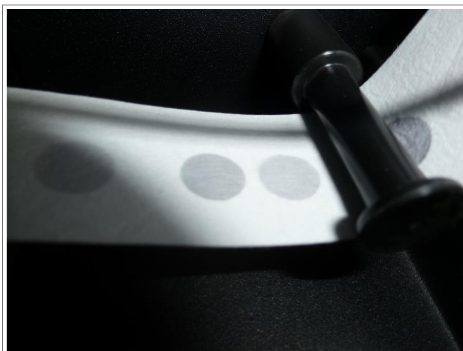
Figure 1: New spot from AE33 (S02-00267) on filter tape.
