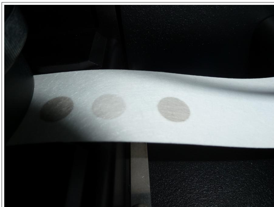
Figure 1: New spot from AE33 (S00-00049) on filter tape.
