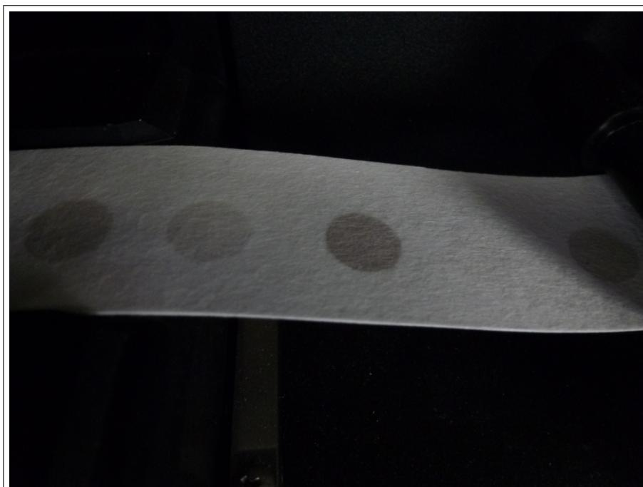
Figure 1: New spot from AE33 (S05-00443) on filter tape.
