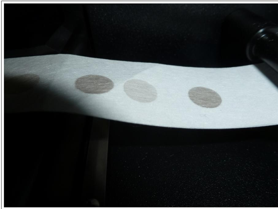
Figure 1: New spot from AE33 (S07-00783) on filter tape.
