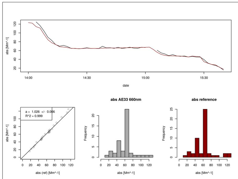
Figure 4: Correlation of absorption from AE33 (S07-00783) and the multi-wavelength absorption reference at 660 nm.
