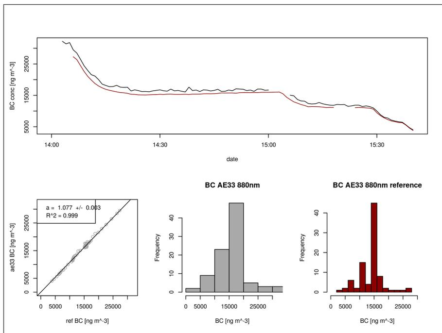
Figure 3: Correlation of eBC coefficient (BC6) from AE33 (S07-00783) and reference AE33.
