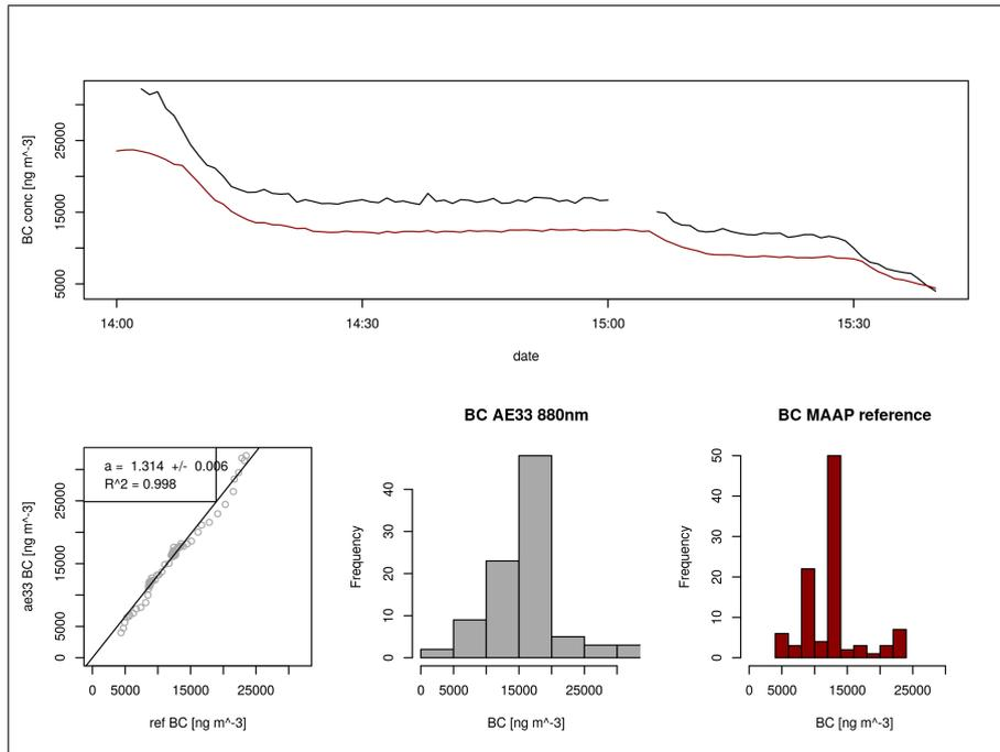
Figure 2: Correlation of eBC coefficient (BC6) from AE33 (S07-00783) and reference MAAP.
