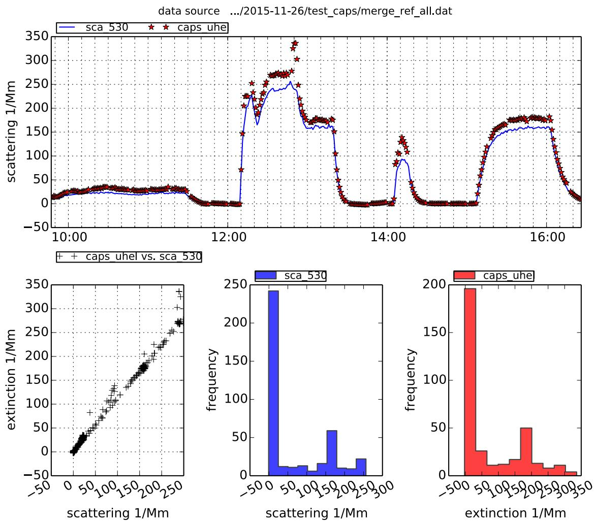
Figure: Inter-comparison to scattering from Nephelometer using ammonium sulphate. Nephelometer data were corrected for scattering.
