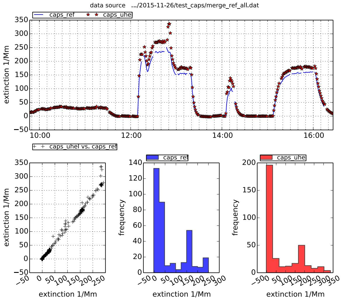
Figure: Comparison to reference CAPS at 530 nm using ammonium sulphate as test aerosol.
