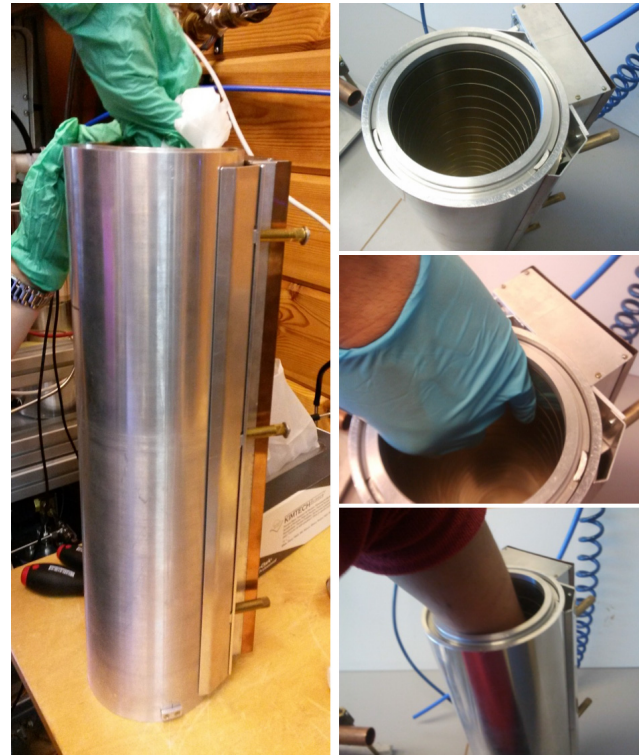
Figure 11. Cleaning electrometer rings by opening the mobility analyzer and wiping with a clean cloth.
